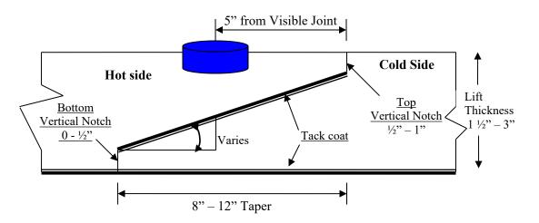
Cores may be obtained daily or weekly. All cores must be cut within 5 calendar days of placement. Any core that is damaged or obviously defective while being obtained will be replaced with a new core from a location within 2 feet measured in a longitudinal direction.
