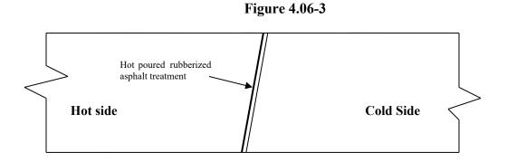
All of the requirements of Method II must be met with Method III. In addition, the longitudinal vertical edge must be treated with a joint seal material meeting the requirements of Section M.04 prior to placing a completing pass. The joint seal material shall be applied in accordance with the manufacturer's recommendation so as to provide a uniform coverage and avoid excess bleeding onto the newly placed pavement.
