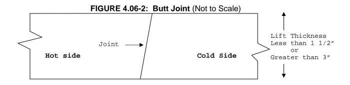
The Contractor shall not allow any butt joint to be incomplete at the end of a work shift unless otherwise allowed by the Engineer. When using this method, the Contractor is not allowed to leave a vertical edge exposed at the end of a work shift and must complete paving of the roadway full width "curb to curb."
