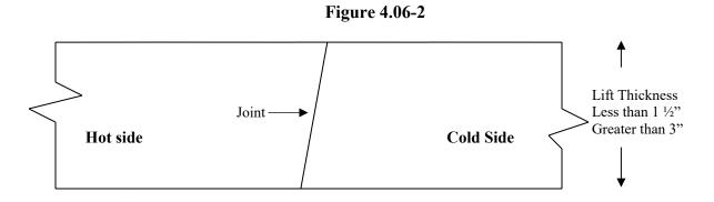
When adjoining passes are placed, the Contractor shall utilize equipment that creates a near vertical edge (refer to figure). The completing pass (hot side) shall have sufficient mixture so that the compacted thickness is not less than the previous pass (cold side). The end gate on the paver should be set so there is an overlap onto the cold side of the joint.
