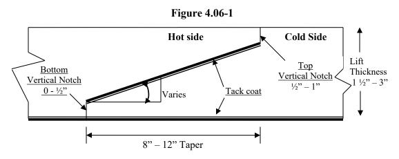
A notched wedge joint shall be constructed, as shown in the figure using a device that is capable of adjusting the top and bottom vertical notches independently and is attached to the paver screed.
